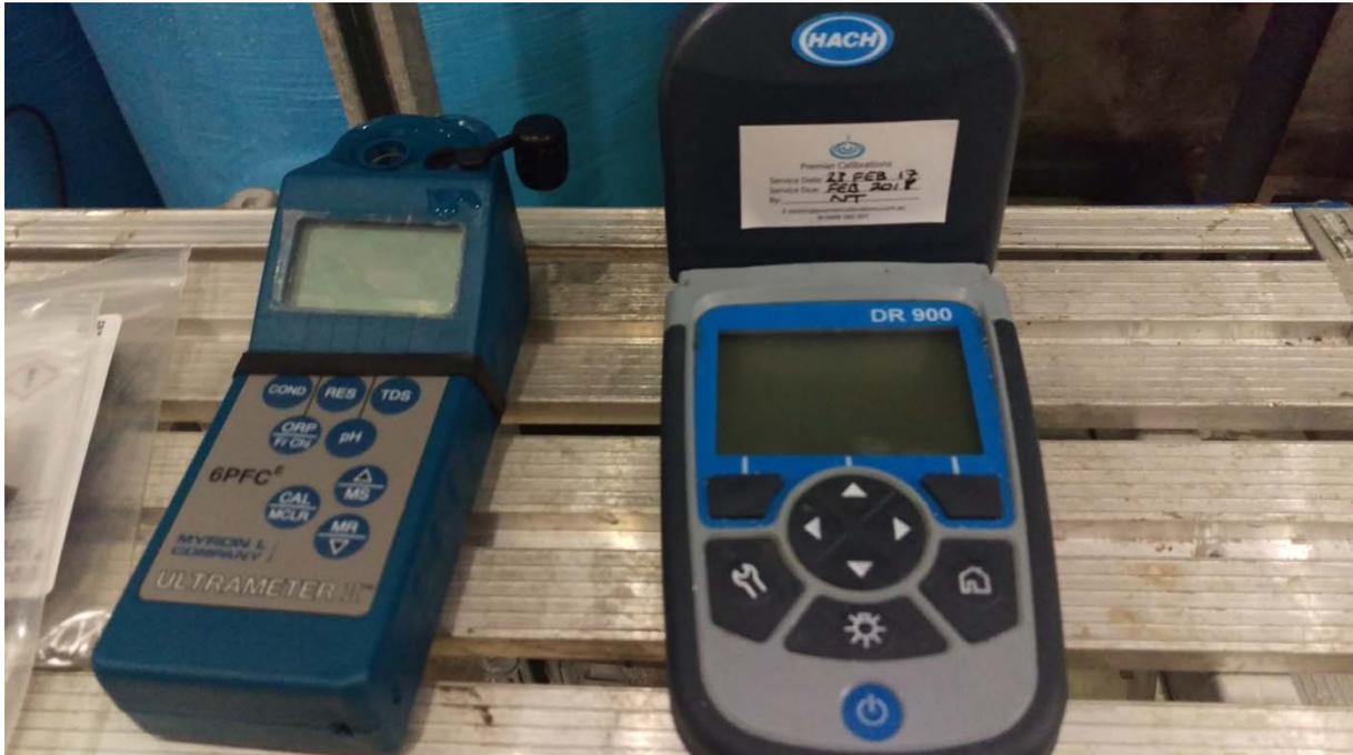
Figure B.1.2 Hach DR 900 Multiparameter Portable Colorimeter showing service sticker.
